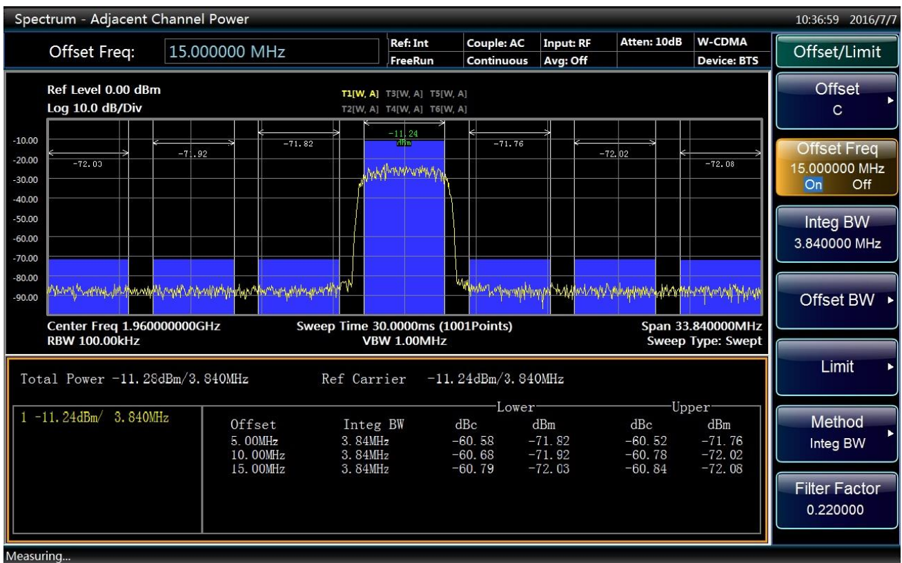
Fig.4.67 Measuring third adjacent channel
