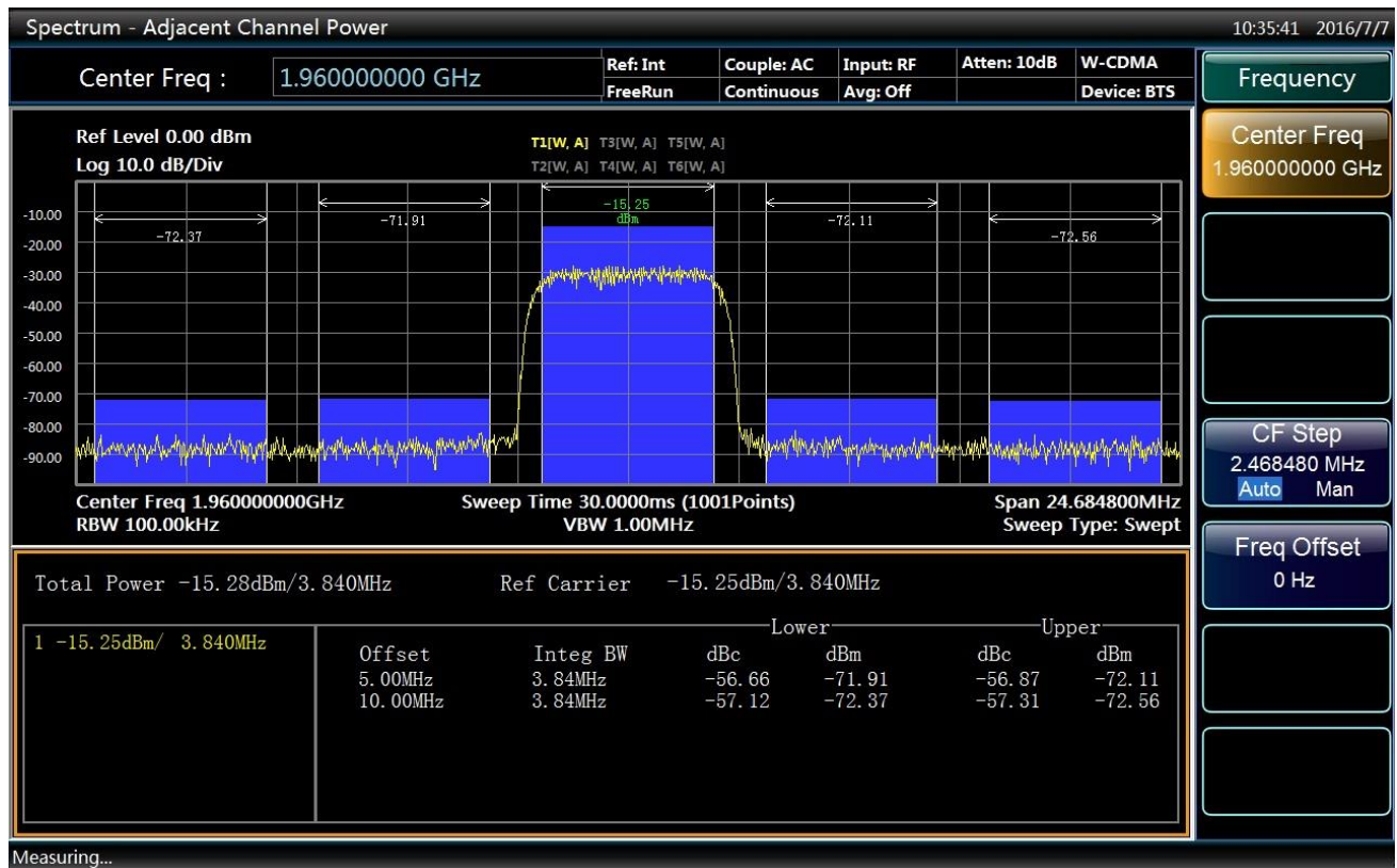
Fig 4.66 Results of Adjacent Channel Power Measurement
